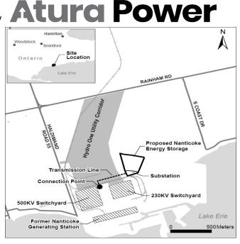
and a system that will convert electrical alternative current (AC) to direct current (DC) for battery storage, as well as ancillary components such as transformers, emergency power, support buildings and transmission connection facilities. The proposed Nanticoke Energy Storage system is located north of the former Nanticoke Generating Station between Haldimand Rd. 55 and South Coast Dr. in Haldimand County, Ont.
