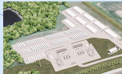
5. Napanee BESS Phase 1 Capacity 250 MW
