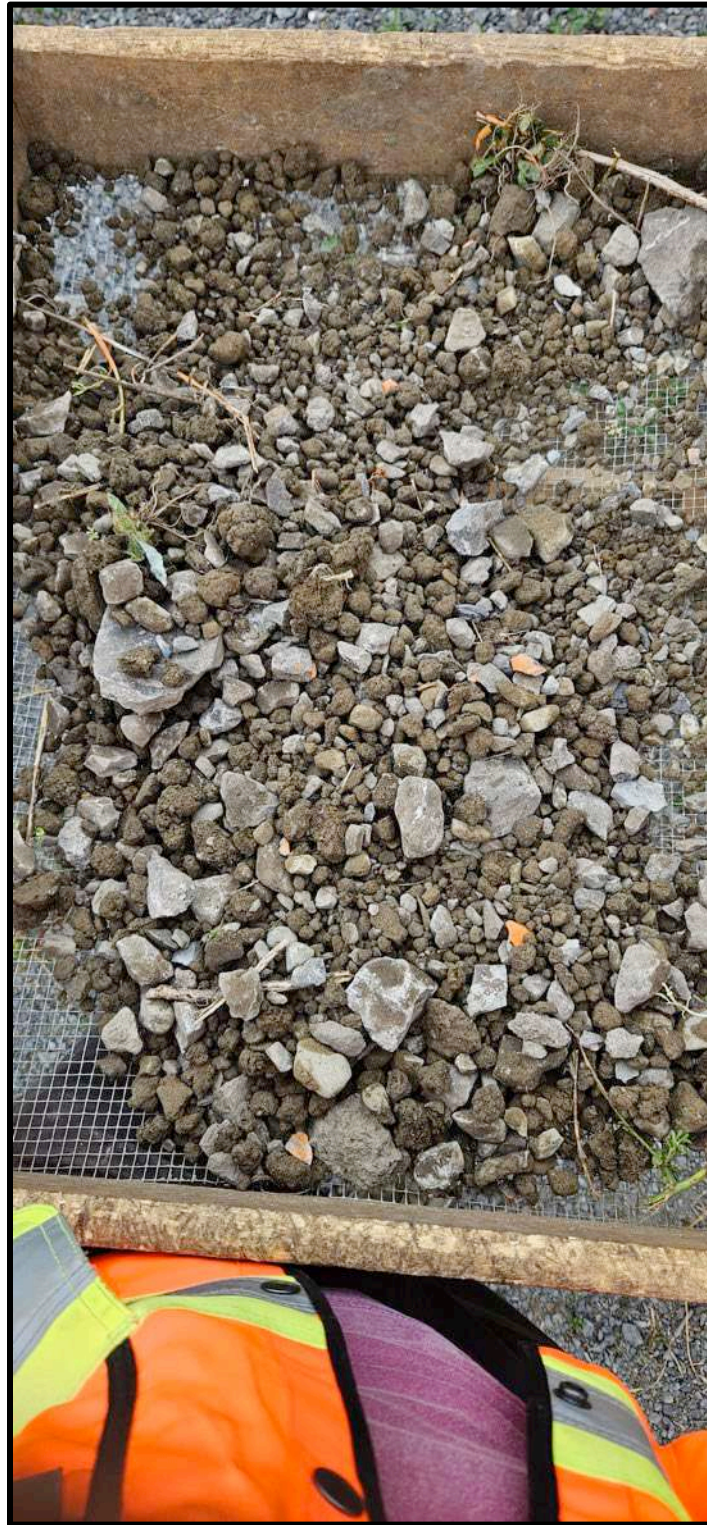
Image 61: View to northeast of sifted soil sample from borehole B-1 in Zone 5, showing abundance of fill (gravel and rock fragments) present in the upper 40 cm.
