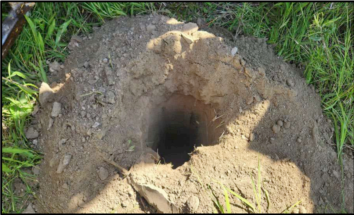
Image 53: View to northwest of soils brought to surface from upper 50 cm of borehole WH-3 in Zone 1. Note predominance of sand and gravel fill.
