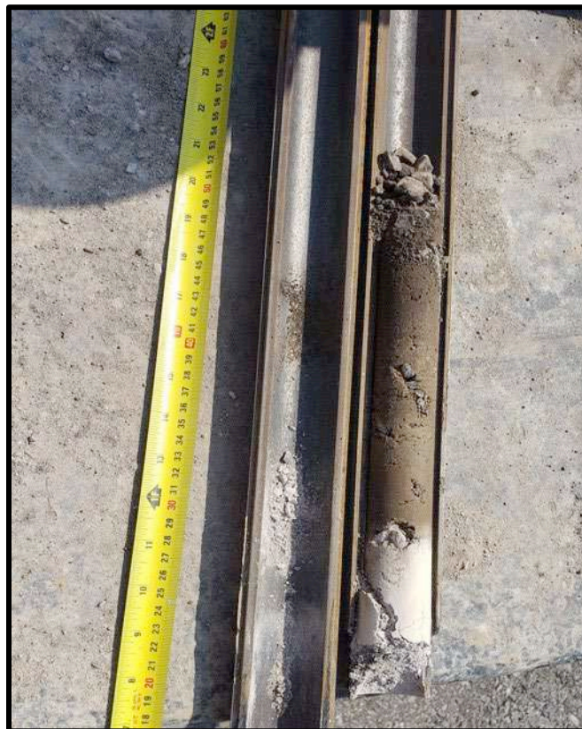
Image 63: View to northeast of soil core from borehole B-3's upper 30 cm, showing presence of concrete, gravel, and sandy fill materials.
