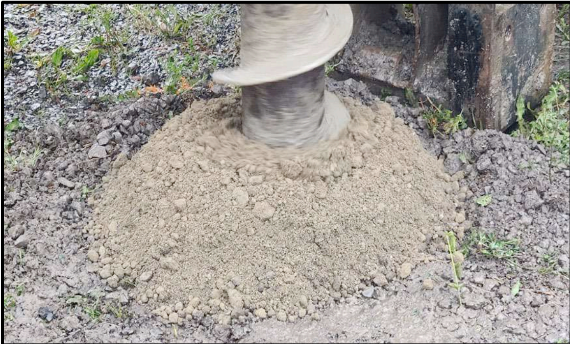
Image 49: View to north of auger bringing soils to the surface during the drilling of borehole WH-1 in Zone 1.
