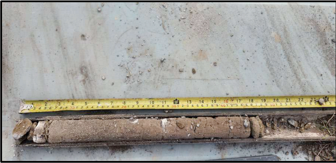
Image 51: View to northeast of core sample from the upper 50 cm of borehole WH-2, showing presence of topsoil mixed with fill materials such as sand and silty clay.
