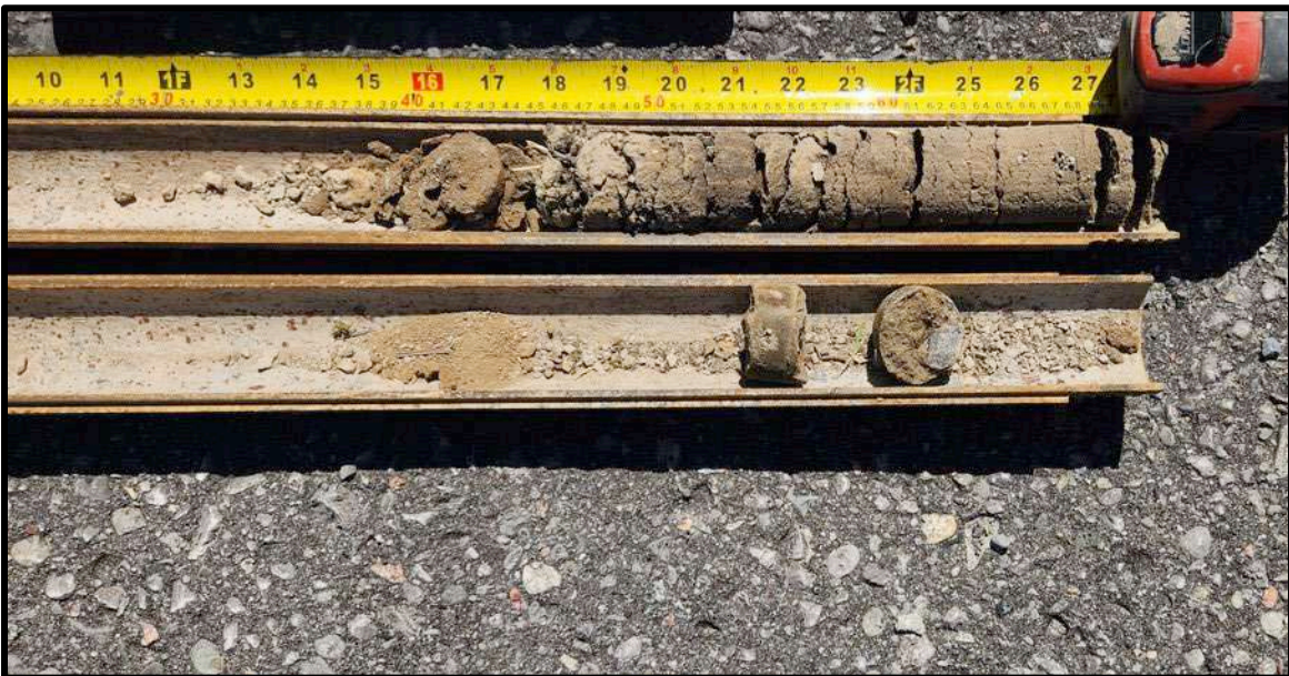
Image 54: View to northeast of core sample from the upper 30 cm of borehole WH-3, showing presence of fill materials such as sand and silty clay.
