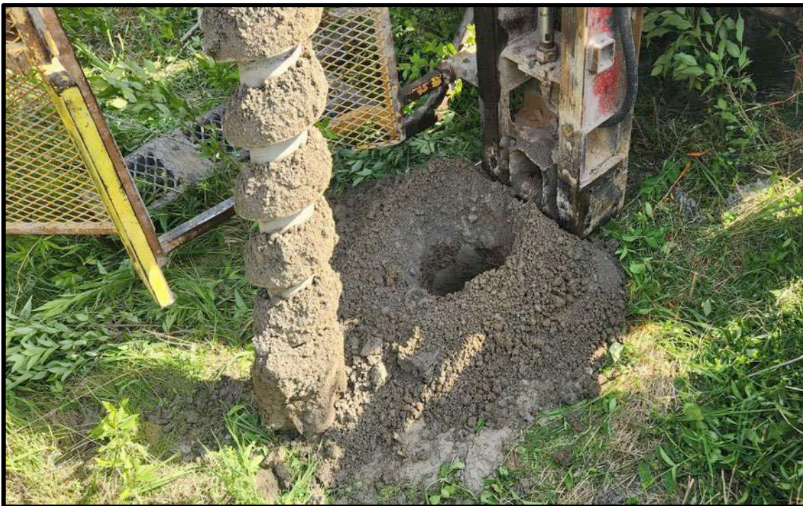
Image 56: View to north of auger and soils brought up from the upper 100 cm of borehole WH-4 in Zone 1. Note mix of topsoil with sand and gravel fill.
